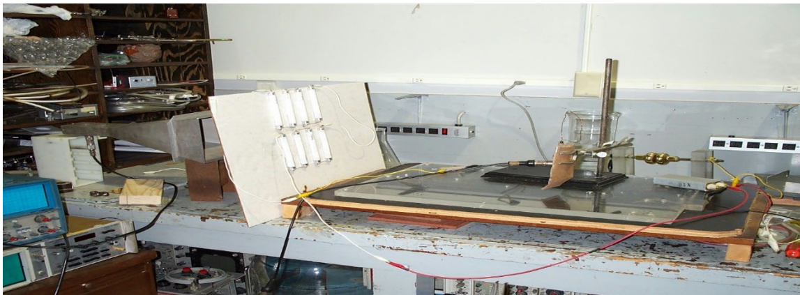
Figure 6. Photograph of the lab setup showing the built plasma dipole reconfigurable FSS with the horn receiver antenna.
