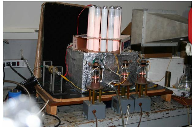
**Figure 6.** Demonstration of a prototype for an intelligent plasma antenna. A ring of plasma tubes operating beyond microwave cut-off surrounds a metal transmitting antenna.
