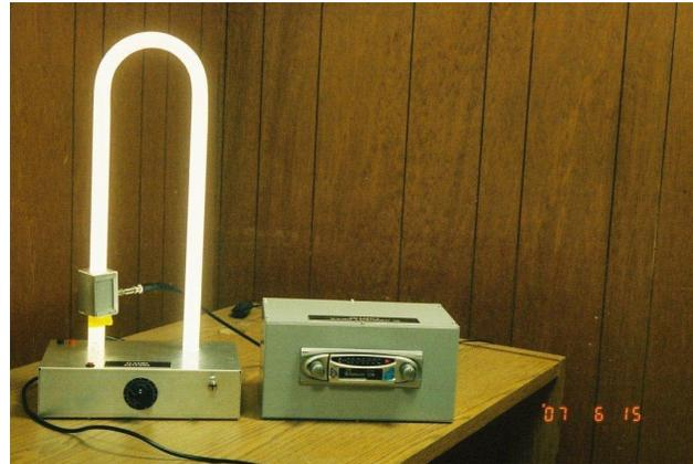
**Figure 5.** A Plasma Antennas connected to a Radio.
