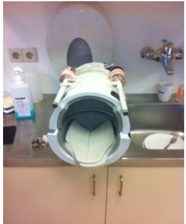
Figure 8. Setup for imaging of the human head with simple fluorescent tubes as plasma antennas.
