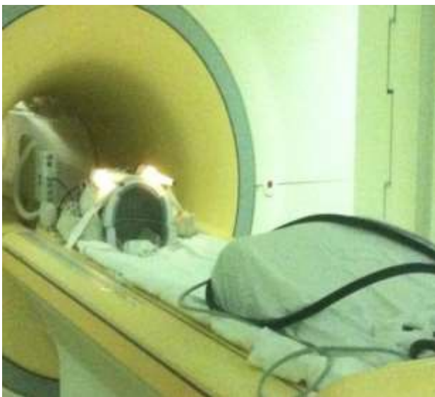
Fig. 6. The setup for imaging of the human head in the MRI machine.
