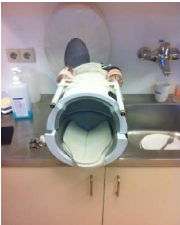
Fig. 5. Setup for imaging of the human head with simple fluorescent tubes as plasma antennas
