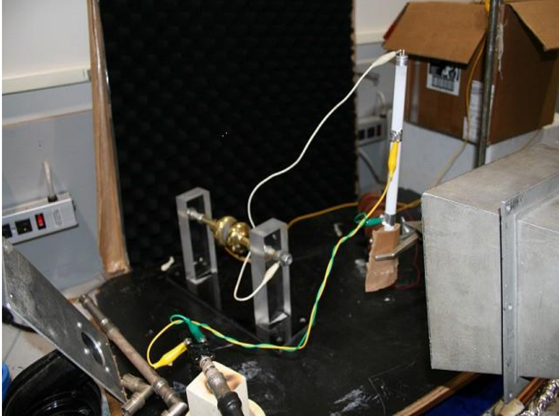
Figure 7.. Experimental setup for scattering electromagnetic waves off of a plasma dipole antenna and sweeping from 100 MHz to 5 GHz. This is an early experiment with early pulsing device.
