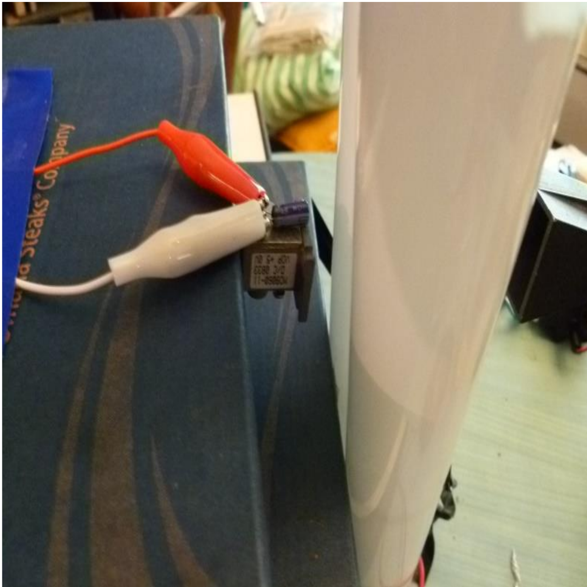
. Plasma focusing experimental setup. Gunn diode 24 GHz transmitter with fluorescent tubes used for plasma beam focus.
