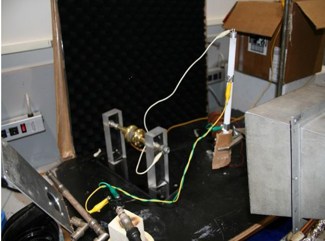
Figure 18.10. Experimental setup for scattering electromagnetic waves off of a plasma dipole antenna and sweeping from 100 MHz to 5 GHz. This is an early experiment with early pulsing device.
