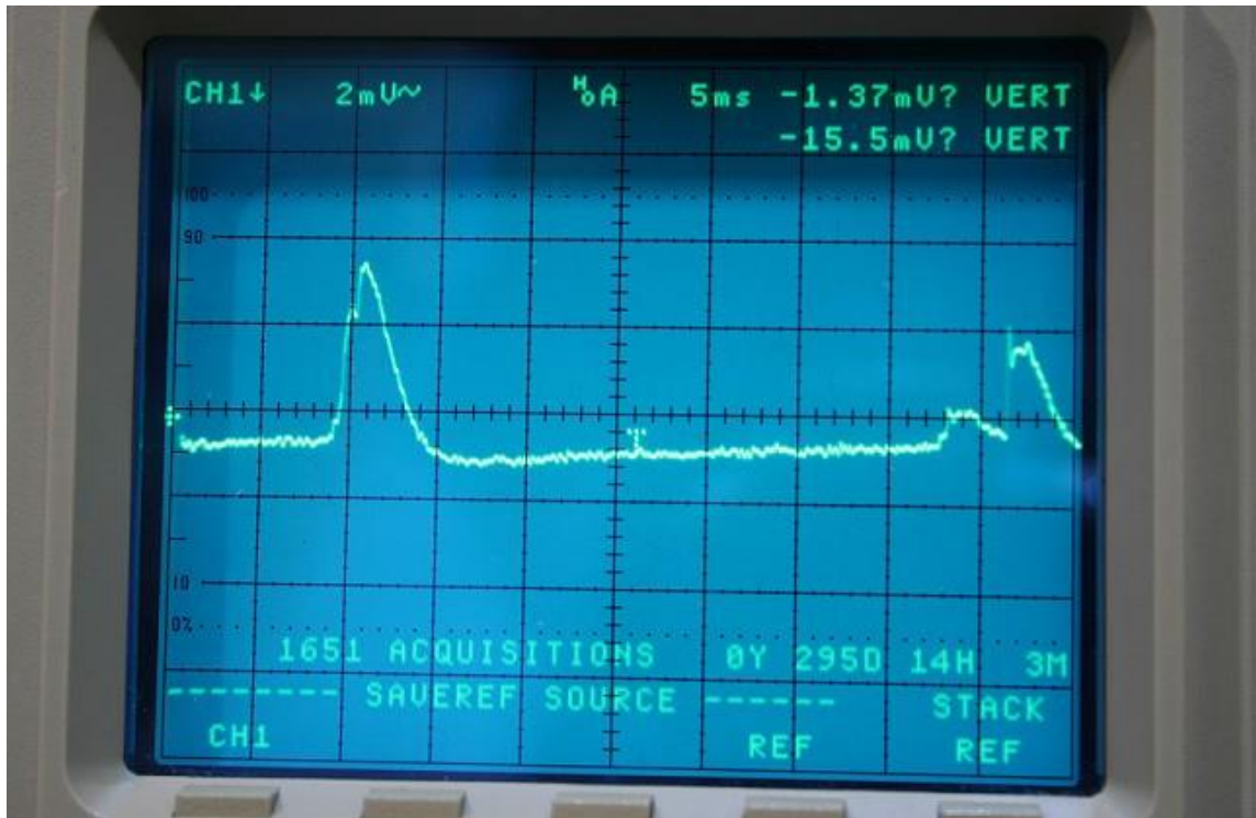
Figure 18.11. Results of the scattering experiment of Figure 18.10. Major and minor resonances are observed as is shown in the simulation of Figure 18.7.
