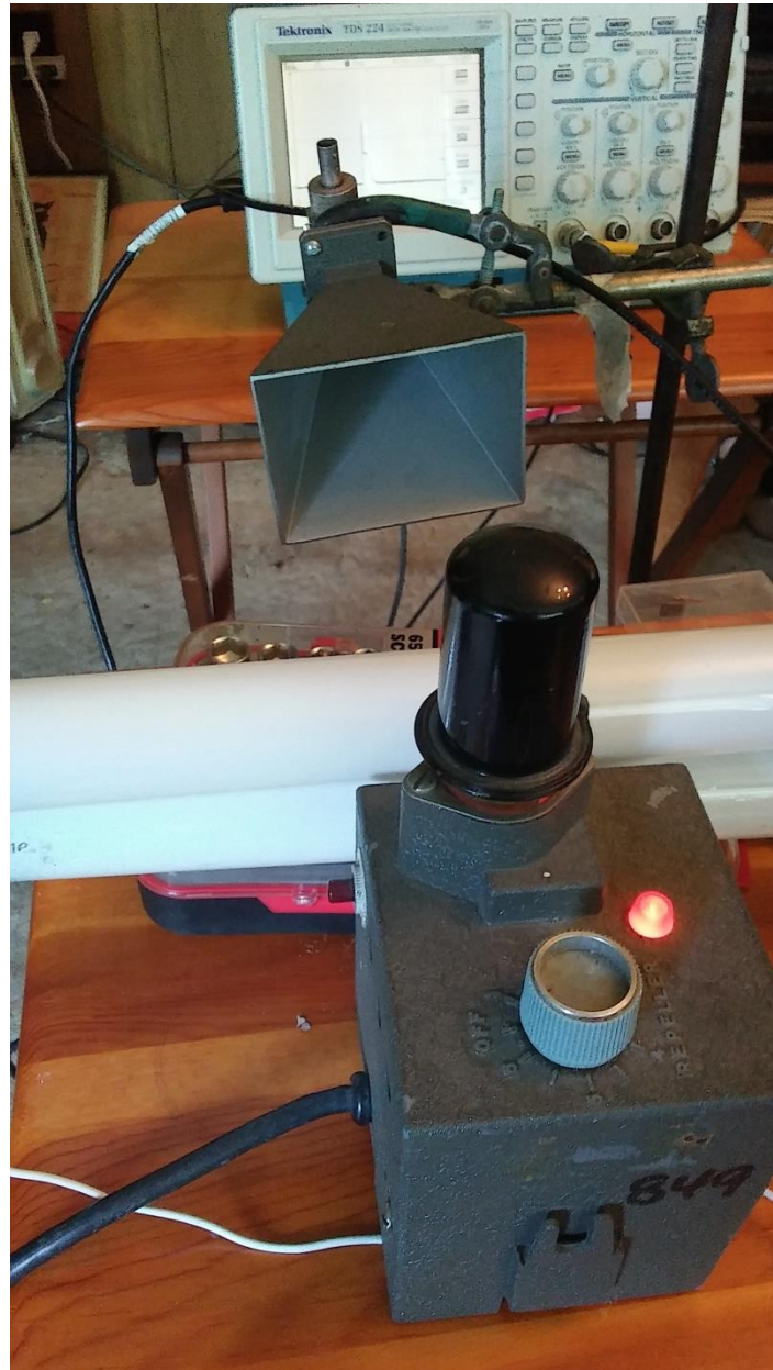
Figure 18.12. Experimental setup for observation of plasma characteristics in the plasma recombination or plasma decay. The Klystron transmits in the X band at 10 GHz. The plasma is pulsed and allowed to recombine or decay and observations are made. Polarization is
