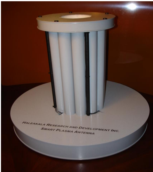
Figure 5. Ruggedized smart plasma antenna RFID reader with engineer prototype.
