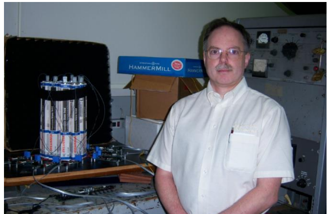
Figure 4. Smart plasma antenna RFID reader with engineer
